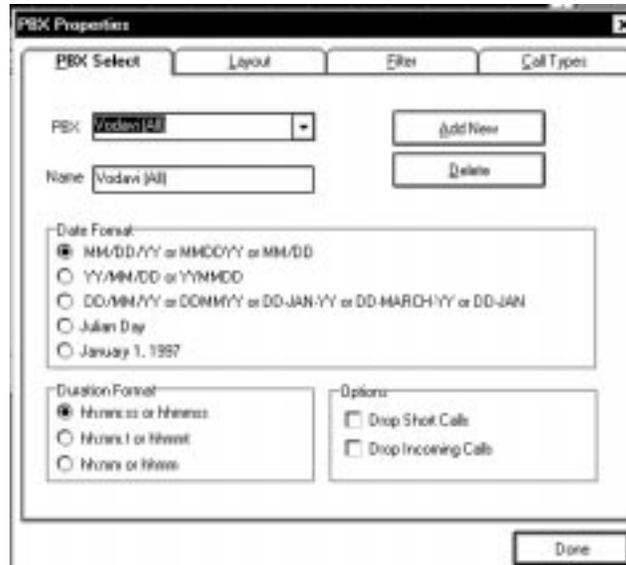
**Figure 2-1: PBX Select Tab (PBX Properties Screen)**
